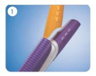
To remove the Geno-Caps™ from the front of the Pen, insert the lip of the pen lid into the groove under the front end of the panel and lever the panel off.
